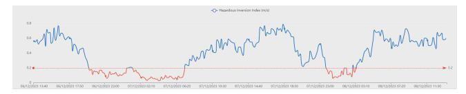
This figure shows the time of a hazardous inversion in the Condobolin district in the last 24 hours – were you spraying around Condo between 11:40pm and 3:10am last night (7<sup>th</sup> Dec) or between 8:10pm and 7:10am the previous night (6<sup>th</sup> Dec) If so, you were spraying during a hazardous inversion and high risk you will have drifted chemical off target! This is ILLEGAL.
