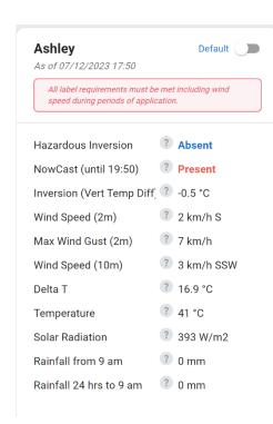
This is what the app looks like when you choose a tower on WAND. If you were spraying now, you could see that a hazardous inversion is imminent within the next 2 hours, so you need to be checking the wand regularly and planning to pull up until the inversion has passed.
