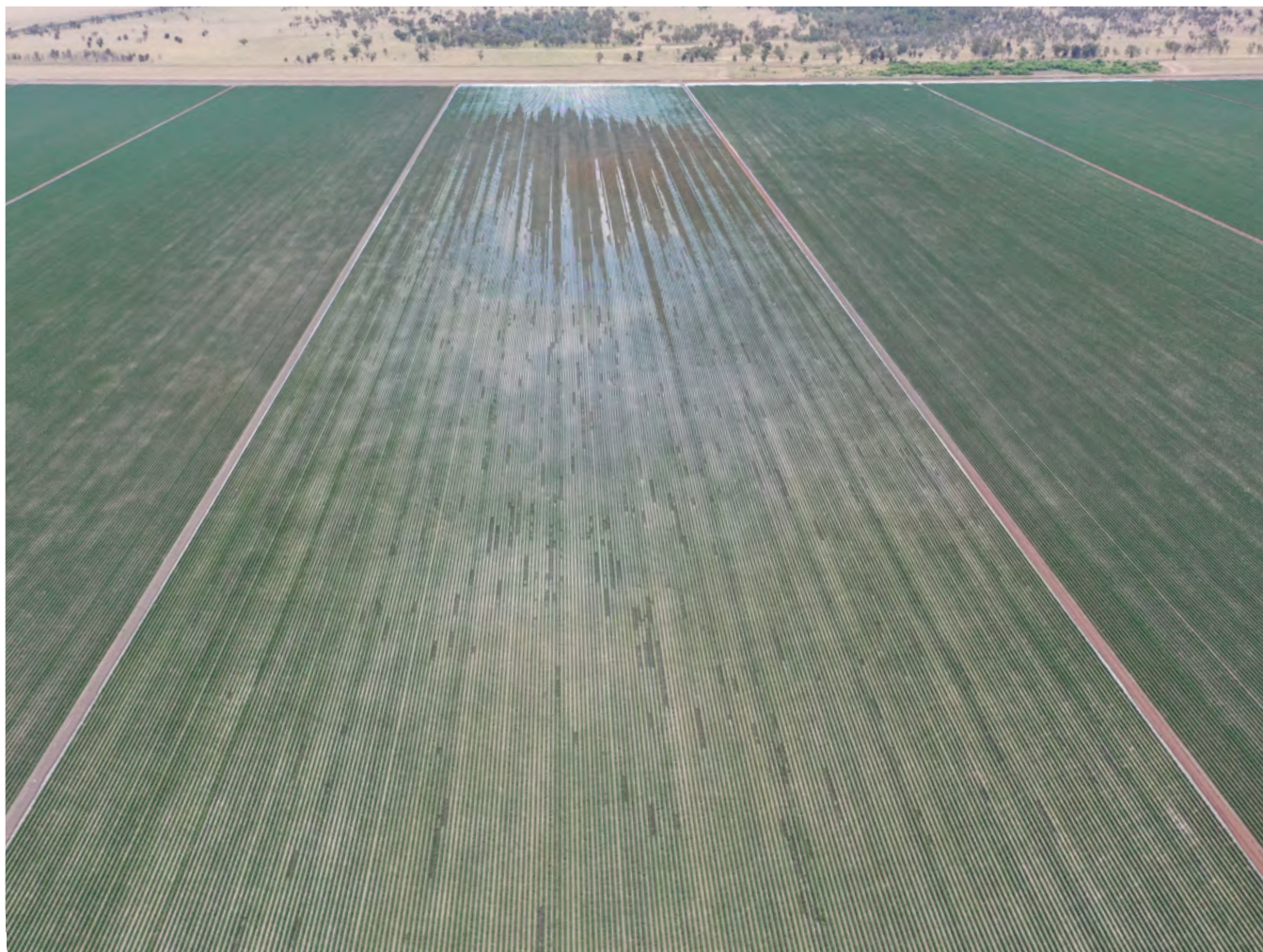
Figure 4: Pipes with Tailwater Backup. Note top of image is tailwater backing up.
