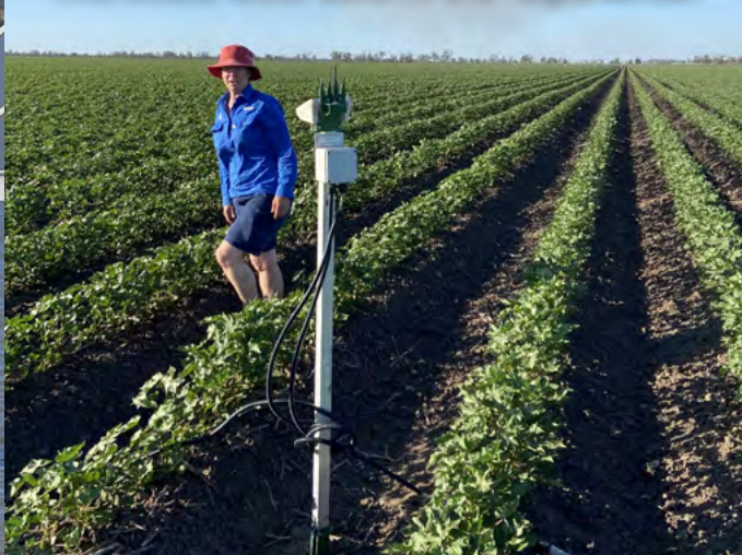
Figure 9: Water level and water advance sensors can help monitor irrigation progress or can be incorporated into remote and automated control. LEFT: Storage water depth sensor. THIS IMAGE: Water advance and height sensor.
