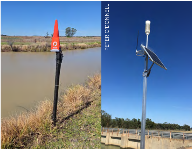
Figure 3: LEFT: Water height sensors can be used for monitoring channel conditions. RIGHT: Weather stations can enhance irrigation decision making.
