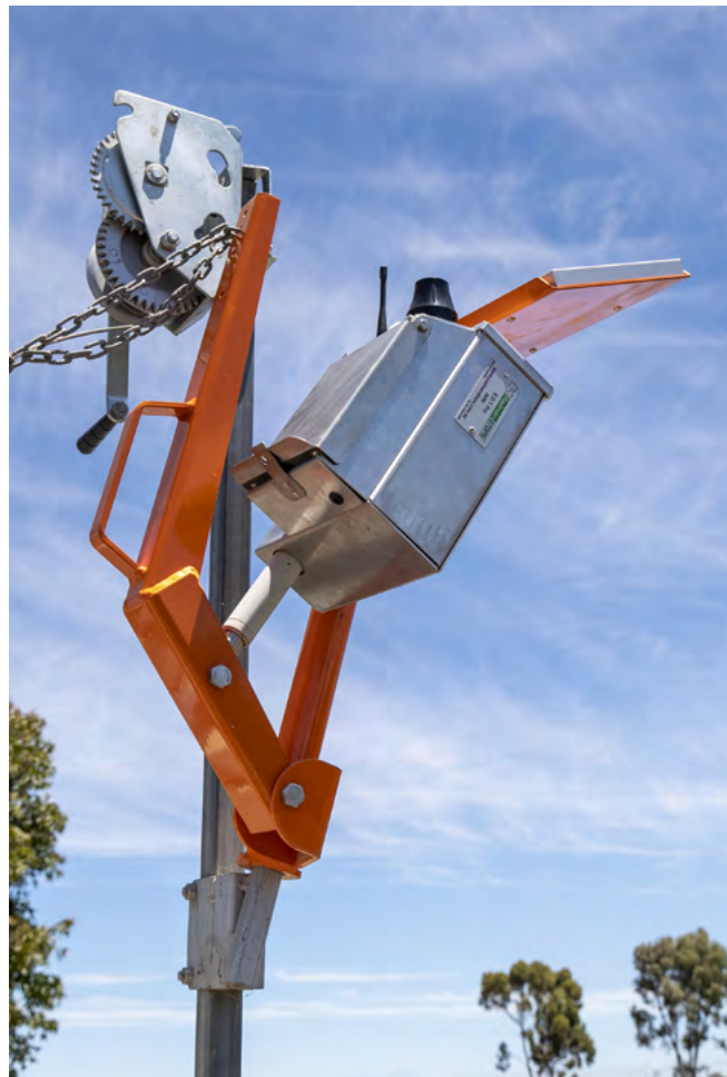
Figure 10: Example of a timer-based controller that can open and close based on pre-programmed commands.
