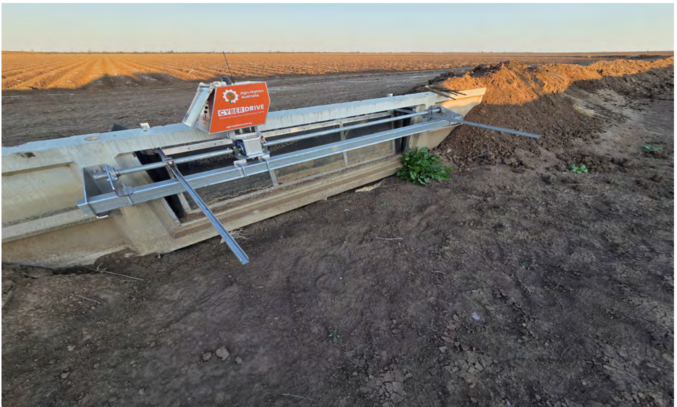
Figure 6: Example of a low-profile (avoids impeding machinery operations) direct-drive mechanism fitted with solar powered controller (top) that can be removed for manual control via cordless drill.
