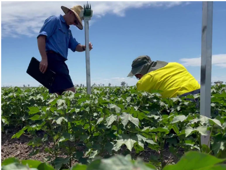
Figure 1: Installing water advance sensors
