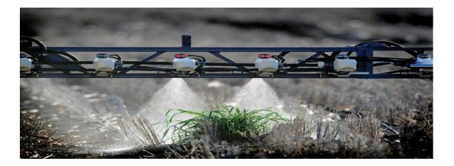
**Caption:** Camera sprayers have increased in popularity with overall big reductions in chemical use in fallow fields. High chemical rates can be applied to individual weeds when a number of nozzles fire. This can have residual chemical carryover effects on the following cotton crop.
